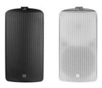
The ES108T is a highly weather-resistant, single 8" 2-way full range loudspeaker, the body is made of engineering plastic injection molding.fitted with one 8" mid-woofer and one 1" HF driver. The system conforms to IP46 international standard. ES108WT is equipped with multi-tap transformer based on ES108, 37.5W/75W/150W/OFF/16? optional.
