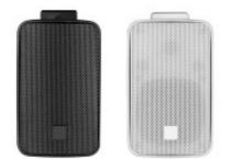
The ES104T is a highly weather-resistant, single 4" 2-way full range loudspeaker, the body is made of engineering plastic injection molding. fitted with one 4" mid-woofer and one 0.8" dome tweeter. The system conforms to IP46 international standard. ES104T black is only available in multi-tap transformer version, ES104BT, 10W/20W/40W/OFF/16? optional.
